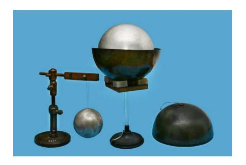
This apparatus was used in Maxwell's determination of the inverse square law of electrostatics in 1877-78. The experiments were carried out with Donald MacAlister and resulted in an improvement by a factor of 1000 in the accuracy with which the inverse square law of electrostatics was known to hold good. This technique used the absence of an electric field inside a conducting spherical shell and was proposed by Henry Cavendish.
