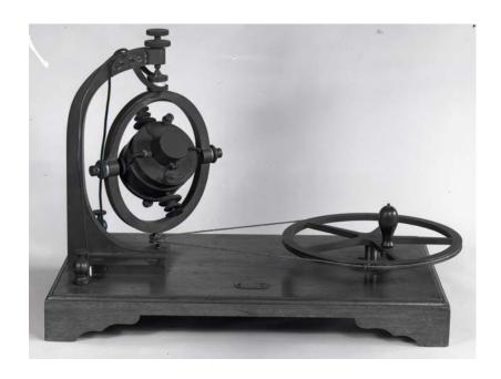
Maxwell's apparatus to measure the inertia of an electric current as it flowed round a current loop. This was one of three experiments Maxwell performed to detect the inertia associated with the flow of current, or the rotational inertia of a magnetic field, none of which showed any evidence for such a phenomenon. These experiments were carried out long before it was understood that electric currents are associated with the flow of electrons.
