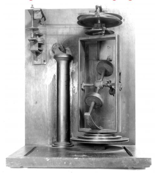
Maxwell's paper of 1868 'On Governors' sets out the theory of control systems and feedback and is regarded as the foundation paper of the field of cybernetics. This governor was needed to control the spinning of the coil in the determination of the ohm. Fleeming Jenkin was one of the leading members of the British Association Committee on electric standards and carried out the first spinning coil experiments with Maxwell.
