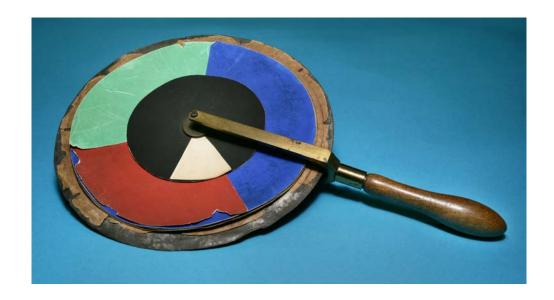
Maxwell did most of his work on the quantitative theory of colour in the time between finishing his BA early in 1854 and starting his research Fellowship at Trinity College in late 1855. The mixing of different amounts of the primary red, green and blue lights could be used to synthesize any colour. The merging of these primary lights was achieved by rotating the disc rapidly. The central black and white sectors enabled a grey comparison light to be synthesized.
