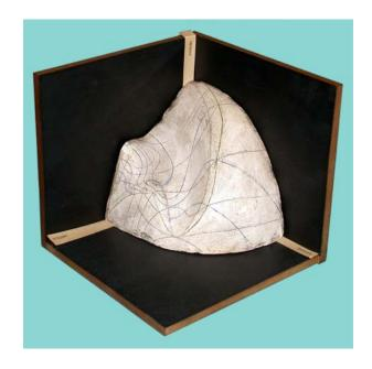
Maxwell's plaster model of Gibbs's thermodynamic surface of water of 1876. The three-dimensional coordinates are volume, entropy and energy. According to classical thermodynamics, the pressure is the tangential slope of energy against volume; the temperature is the tangential slope of energy against entropy. The three-dimensional model also shows the transition points between the solid, liquid and gaseous phases of water.
