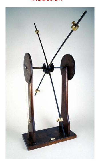
Maxwell's mechanical model of electromagnetic induction. The flywheel is acted upon by two forces at different locations on the axis of the flywheel: these forces are the analogues of electric fields. When one of the forces is changed, this change is communicated to the other force. The equations describing the net changes in force acting upon the flywheel are of exactly the same mathematical form as electromagnetic induction.
