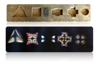
Five pieces of strained glass (from left to right: triangle, square, rectangle with side arcs, cross and circle) observed by Maxwell through a polarizing filter.
