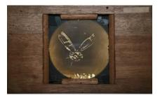
With Maxwell's determination of the three primary coloured lights needed to synthesise any colour, he photographed a tartan ribbon on three plates through red, green and blue-violet filters. The three negative slides are shown above. Three positive plates were produced and the projected images were superimposed through the same filters in a demonstration at the Royal Institution in 1861 When these images were combined, a fully-coloured image was produced.
